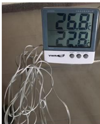
Picture 3-2: Thermometer that can be mounted on a 2 meter stick.
