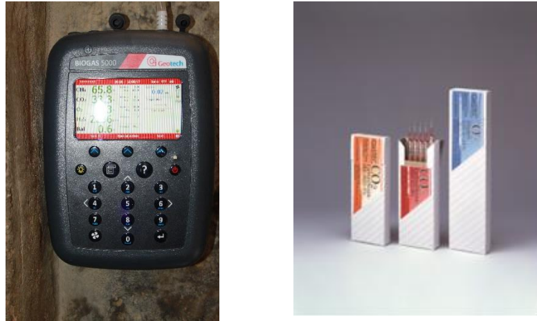
Picture 3-1: Geotech 5000 gas analyser and simple one time use test tubes
