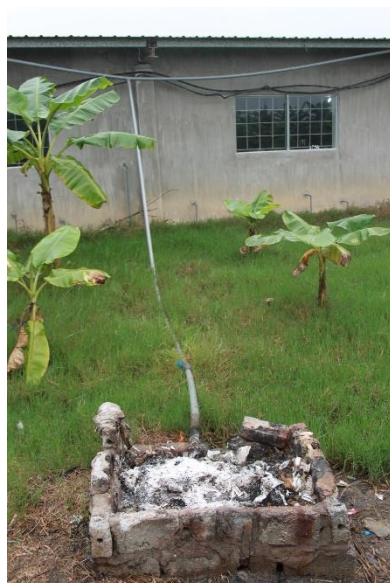
Picture 4-2: a) Simple self-made flaring system in Nam Dinh. b) Heating lamp for piglets running on biogas in Phu Tho.
